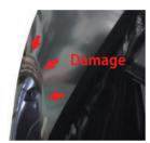
Working with a hammer & dolly will cause more damage.
